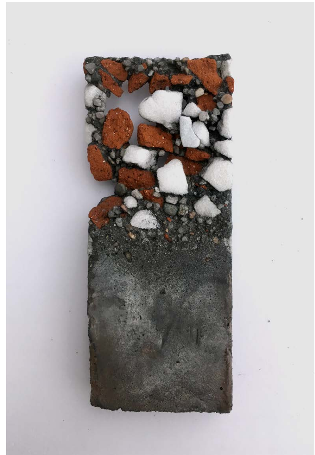
Fig 14, Sample of sandblasted concrete. The aggregates are red bricks (ceramic), marble and sand by Davide Ronco. Copenhagen, DK 2017 Photo: Davide Ronco
