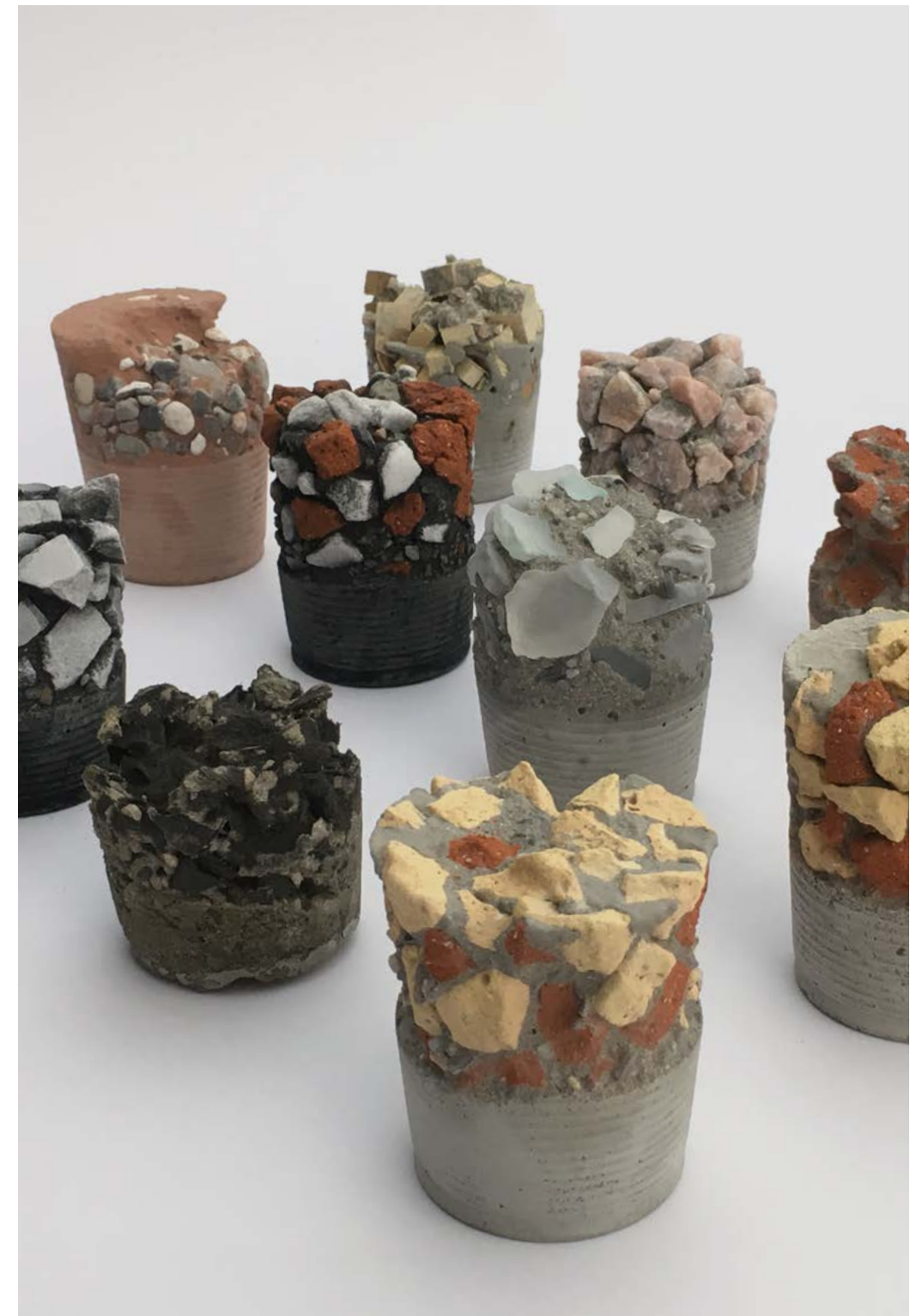
Fig 15, Concrete samples made with different aggregates: ceramic, glass, mdf, wood, stones, common quartz, marble by Davide Ronco. Copenhagen, DK 2017 Photo: Davide Ronco
